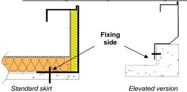
Any other location for fixing may cause water leakage
